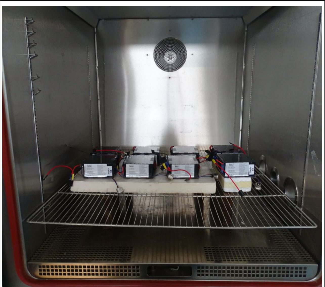
Fig. 2.2 Batteries in T.2 Ref.1 and Ref.2b, §7.2.2 Ref. 2a Test setup (Thermal test, case stress)
