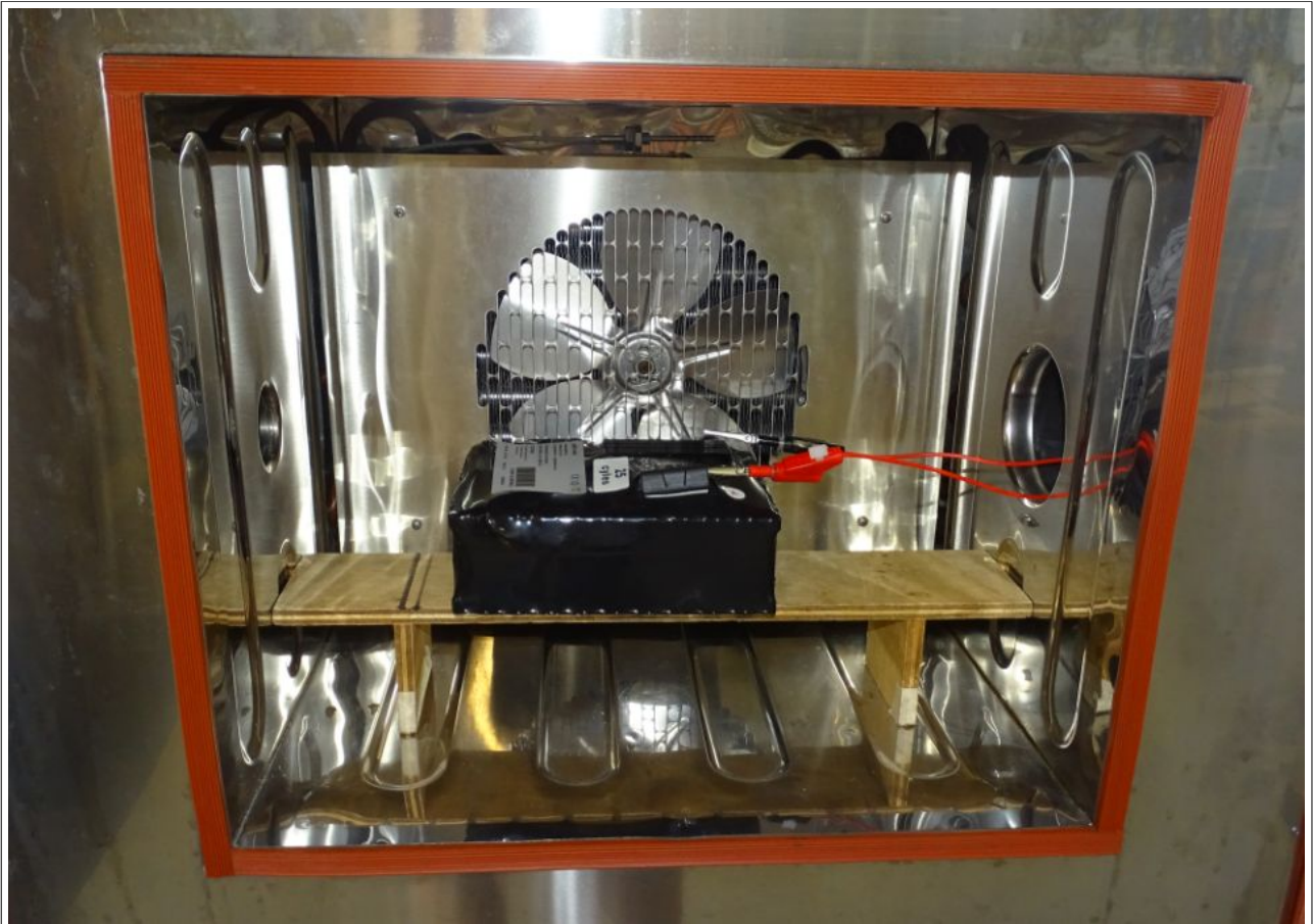
Fig. 2.6 Battery in T.5 Ref.1 and Ref.2b, §7.3.2 Ref. 2a Test setup (External short circuits)
