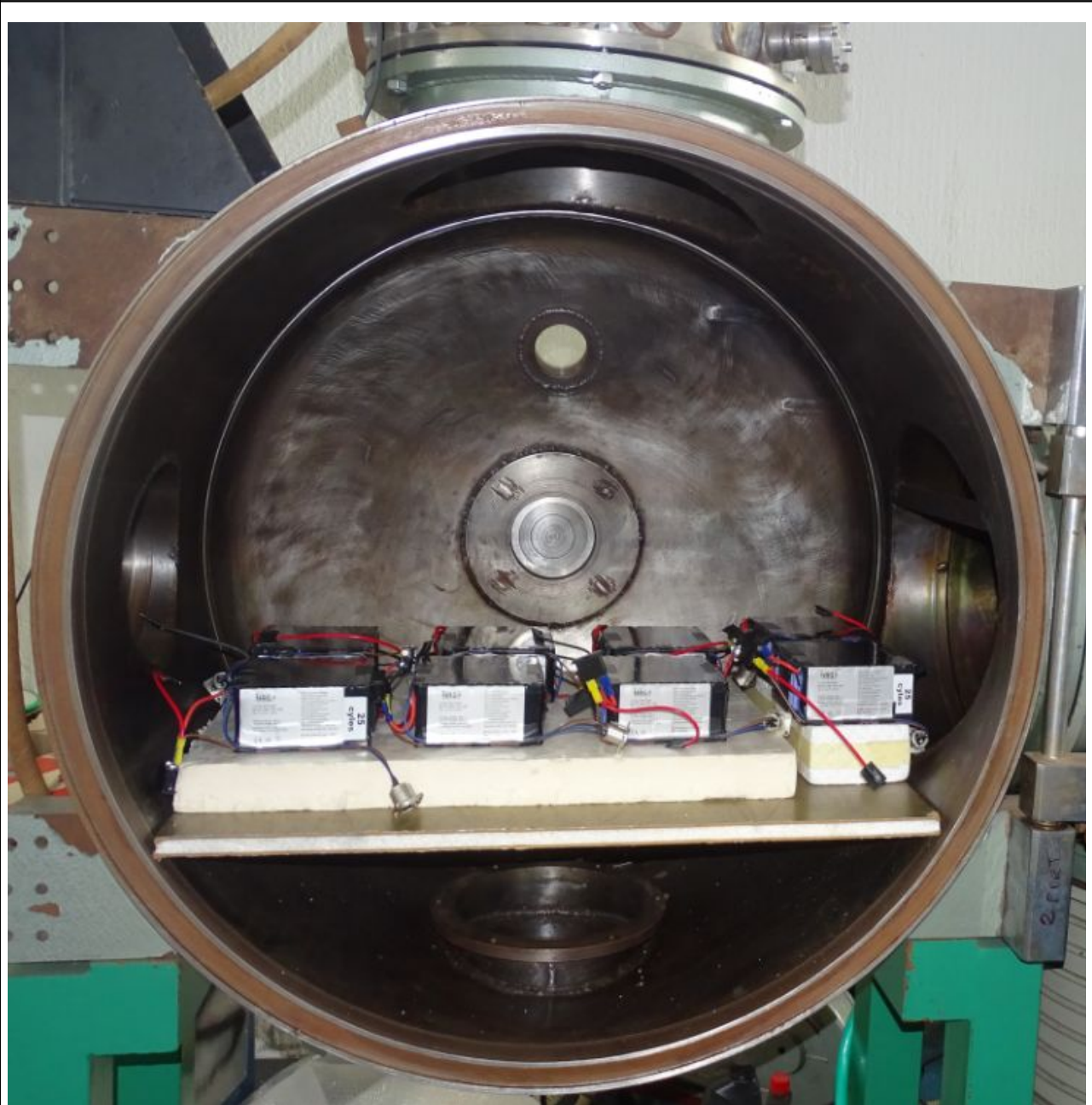
Fig. 2.1 Batteries in T.1 Ref.1 and Ref.2b Test setup (Altitude Simulation test)
