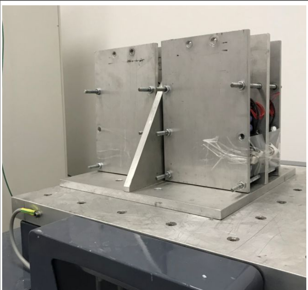
Fig. 2.5 Battery in T.3 Ref.1 and Ref.2b , §7.3.8.1 Ref. 2A and T.4 Ref.1 and Ref.2b, §7.3.8.2 Ref. 2A Test setup (Vibration/Shock test X-Axis)
