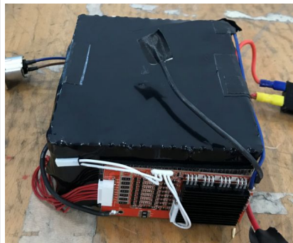
Fig. 2.8 Battery in free fall Test setup, before and after test (Free Fall)
